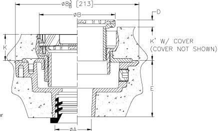
Minimum K Dimension is Only Possible with -LR Option when using 6" [152] or 8" [203] Strainer
